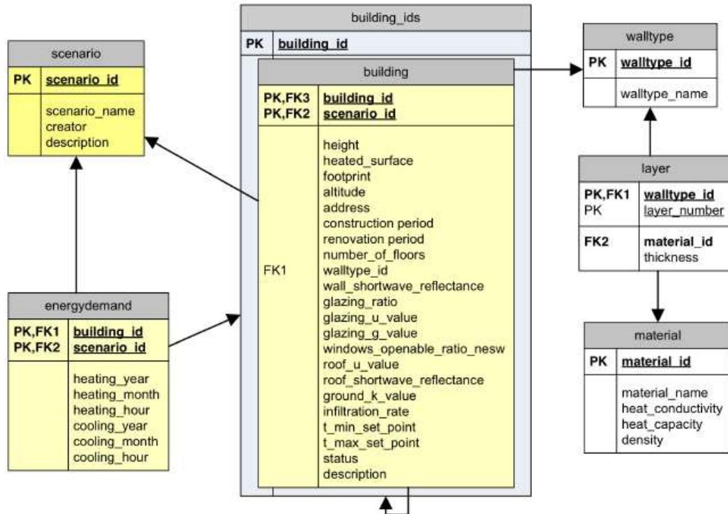
**Figure 2.8: Schema of the CitySim database data model**
