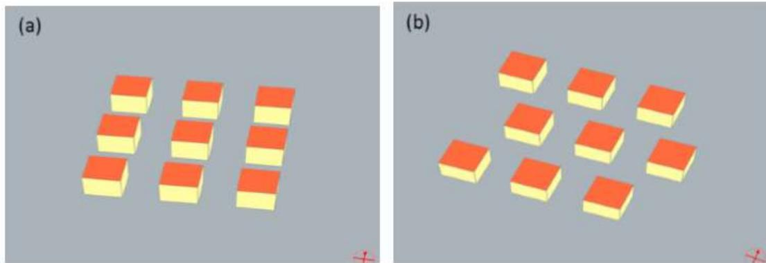
**Figure 2.7: (a) Aligned and (b) staggered building scenarios**
