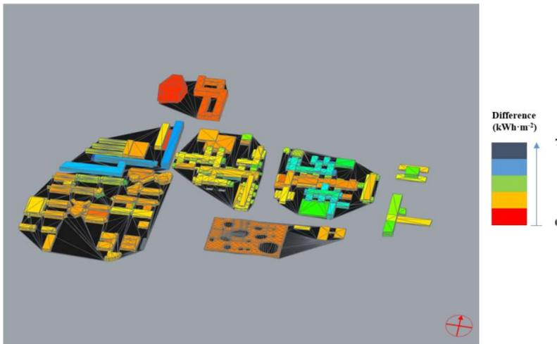
**Figure 2.13: Cooling demand difference for the campus of EPFL for 2009 (Without and with CIM)**
