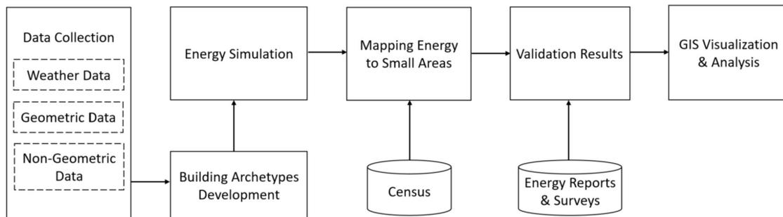
**Figure 2.3: Methodology for GIS-based residential building energy modelling**
