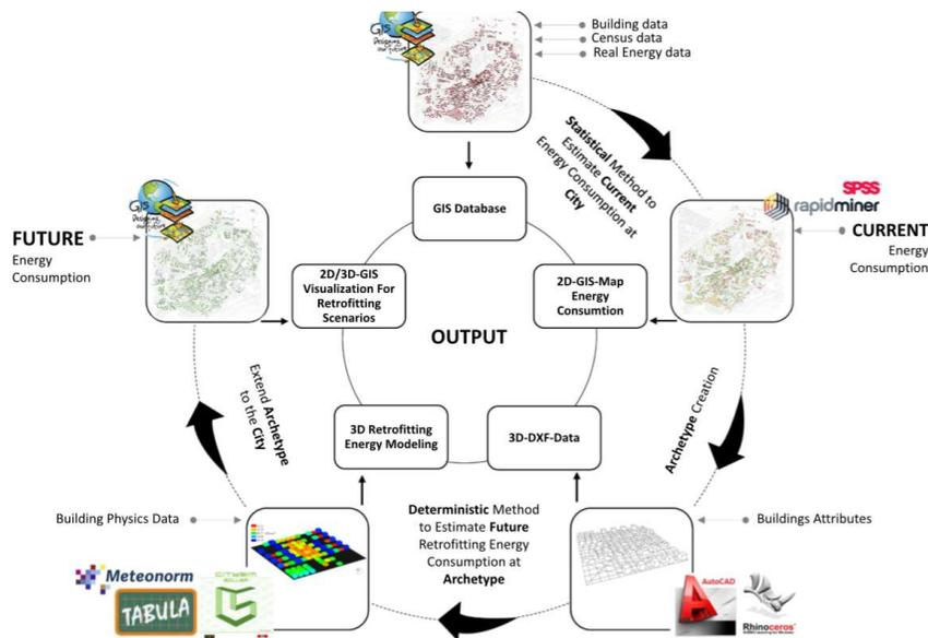
**Figure 2.5:** Flowchart explaining the methodology for creating and using the archetype (Source: Cities, 2019)
