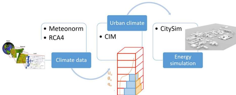
**Figure 2.1: Illustration of simulations flow (CIM – Canopy Interface Model)**
