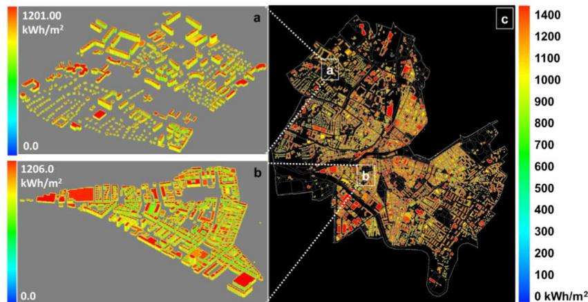
**Figure 2.6: Annual mean solar radiation in KWHm<sup>-2</sup> of building roofs and facades in Geneva using CitySim**
