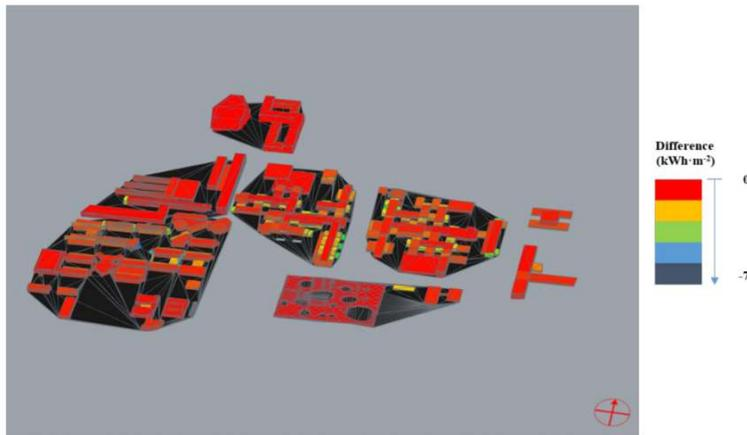
**Figure 2.12: Heating demand difference for the campus of EPFL for 2009 (Without and with CIM)**
