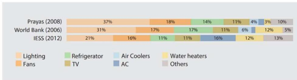
**Figure 1.7: End-use contribution to total consumption of electricity in India**
