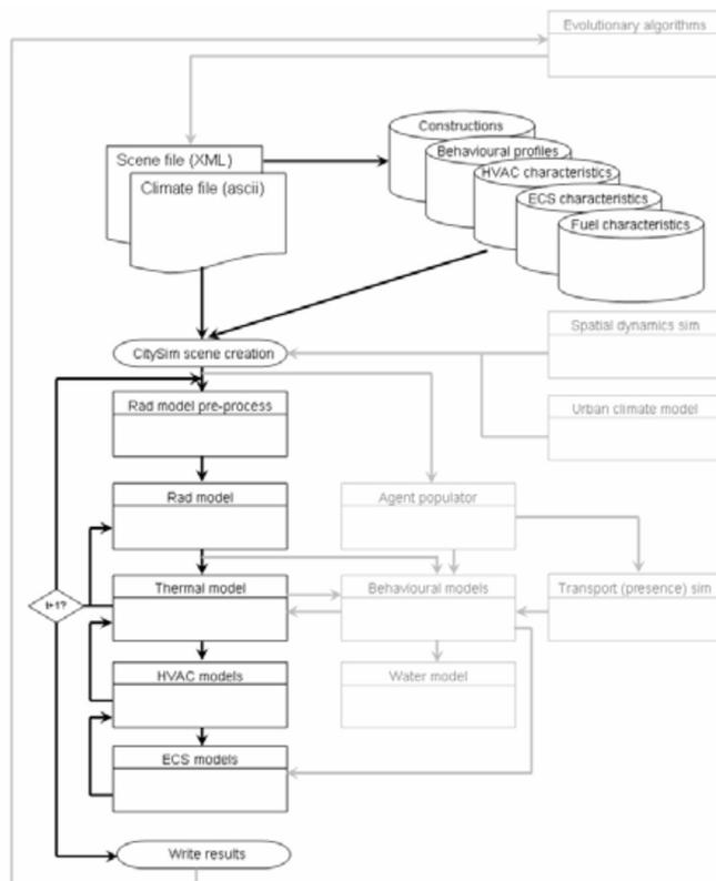
**Figure 2.2: Conceptual structure of CitySim**
